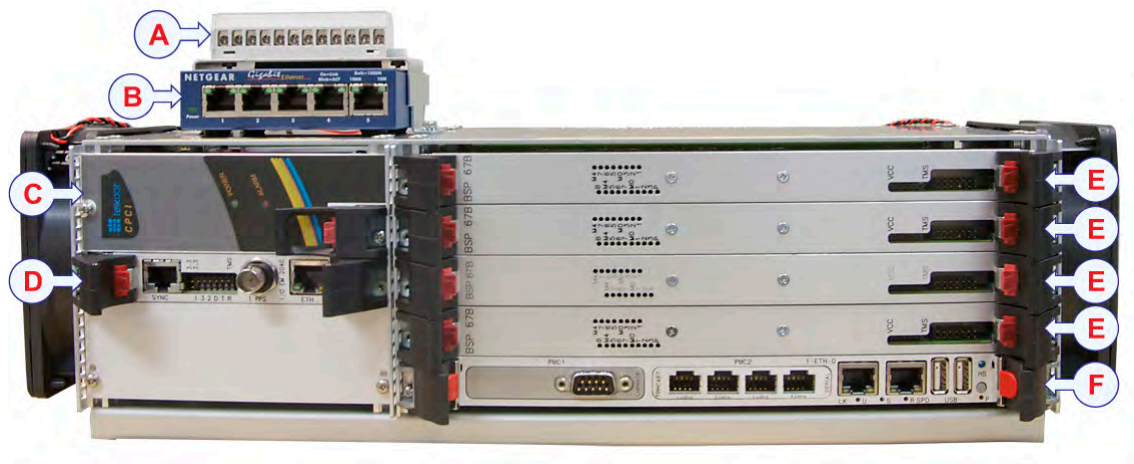
Figure 53 Cylinder AUV processing unit inner assembly
