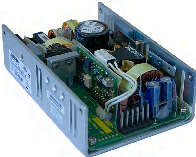
Figure 21 48 VDC power supply
