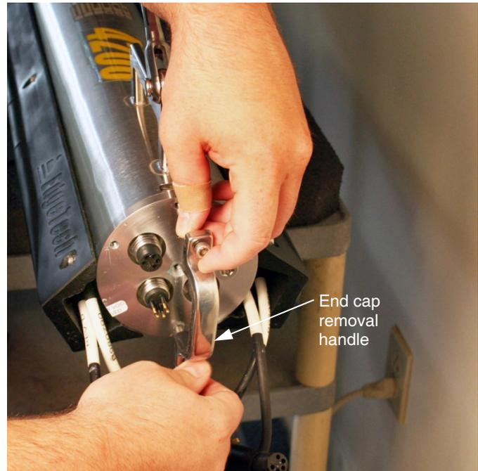
**Figure 5-8: Attaching the End Cap Removal Handle**
