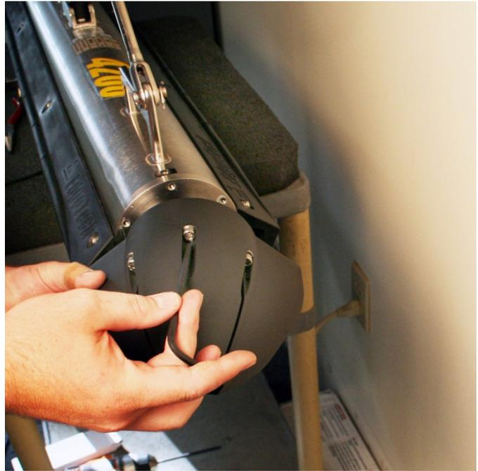
**Figure 5-4: Removing the Tail Cone**
