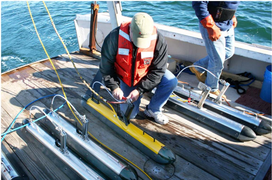
**Figure 1-1: 4200 Series High Definition Dual Frequency Side Scan Sonar Systems being Deployed**
