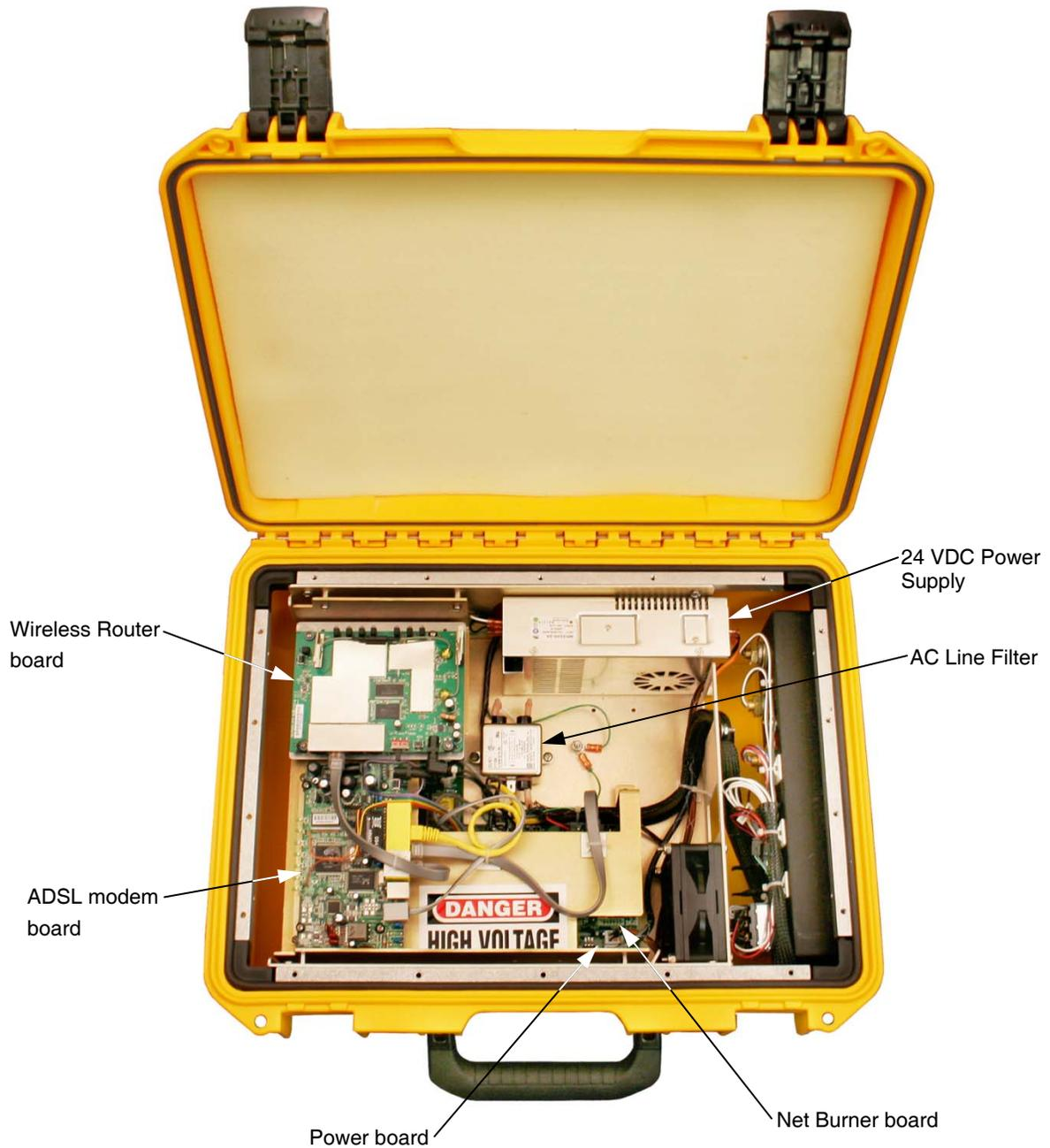
Figure 4-6: 4200-P Portable Topside Processor Chassis
