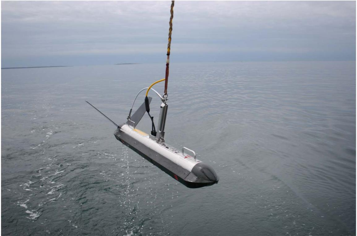
**Figure 3-13:** 4200-MP Tow Vehicle being Deployed
