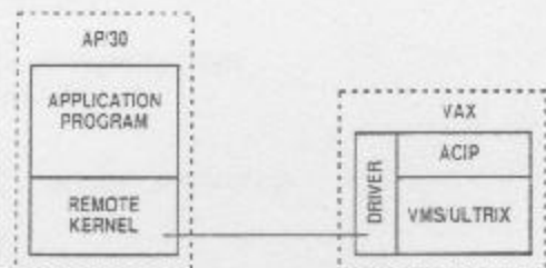
Figure 2: The AP/30 gives users the software they need to maximize the available processing power. Motorola's 88000 is supported by optimizing compilers. Avalon's Central Interface Program (ACIP) provides transparent OS service access to applications running on the AP/30. A local operating system, the Remote Kernel, handles all application system service requests that would normally (if the application were running on an unaided VAX) be handled by VMS.
